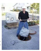
Micro Sam Ex. The control unit can handle flow, volume event or time proportional sampling and is IP65 rated.
