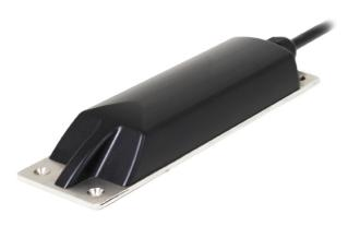
The BELUGA<sup>™</sup> is the newest ultrasonic Doppler area/velocity flow meter sensor for open channel flow measurements from Flow-Tronic. The new sensor combines advanced digital Doppler ultrasonic velocity sensing technology with most modern and powerful DSP processor technology allowing real-time spectral analysis of the velocity distribution through the cross-sectional area.
